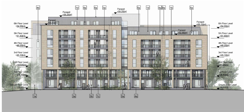
South Elevation - Block 5 Scale 1:200 @A1
