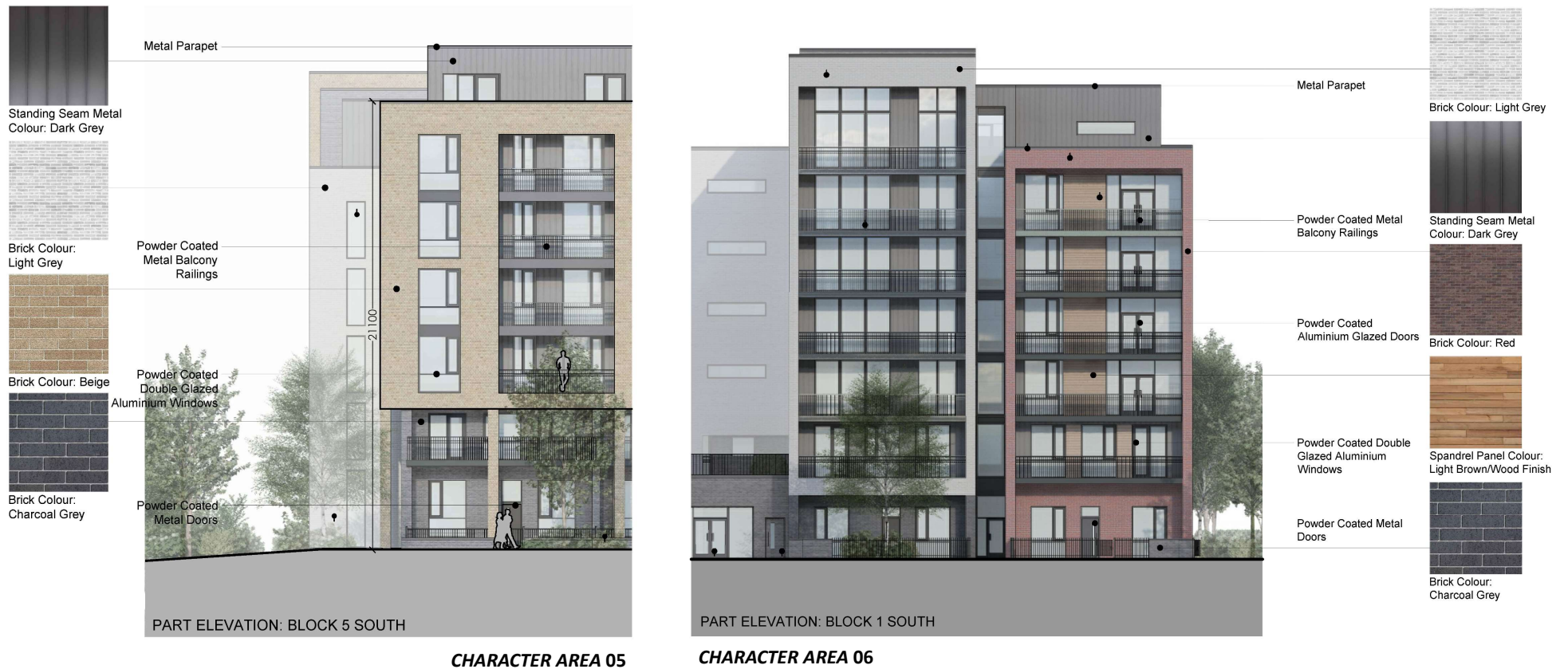
Fig . 01 – Part Elevations outlining Material and Colour Palettes for the different character areas
