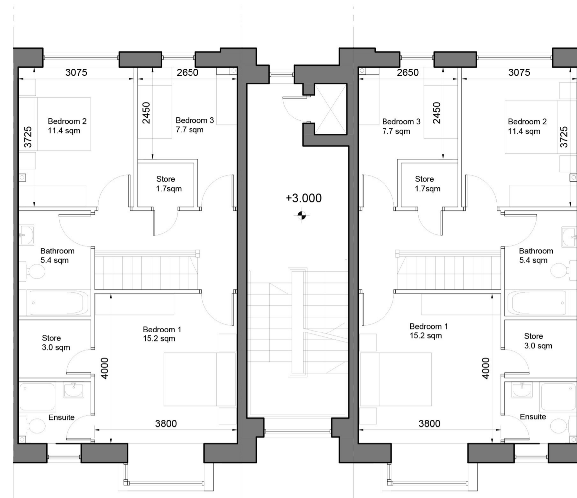
Typical Duplex Type 2A First Floor Plan Scale 1:100@A1
