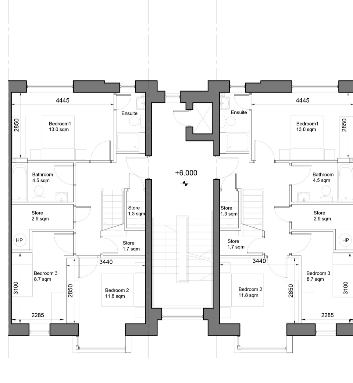
Typical Duplex Type 2B Second Floor Plan Scale 1:100@A1
