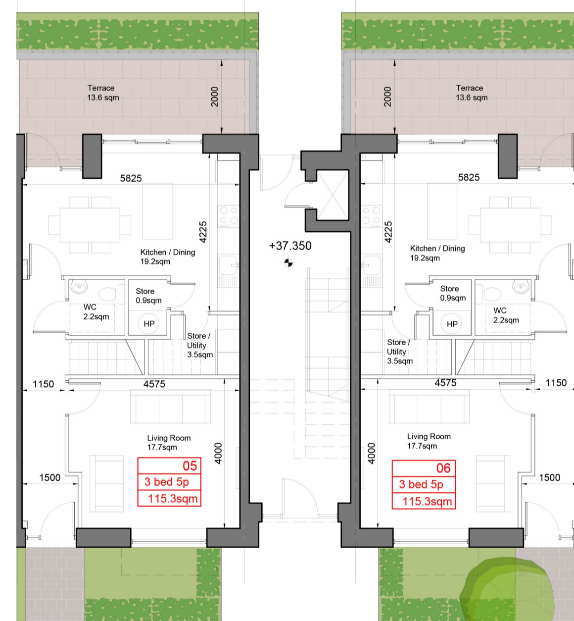
Typical Duplex Type 2A Ground Floor Plan Scale 1:100@A1
