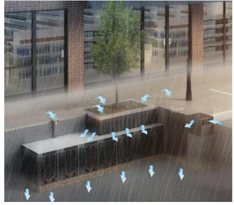
Figure 9.8 Typical Roadside Tree Pit
