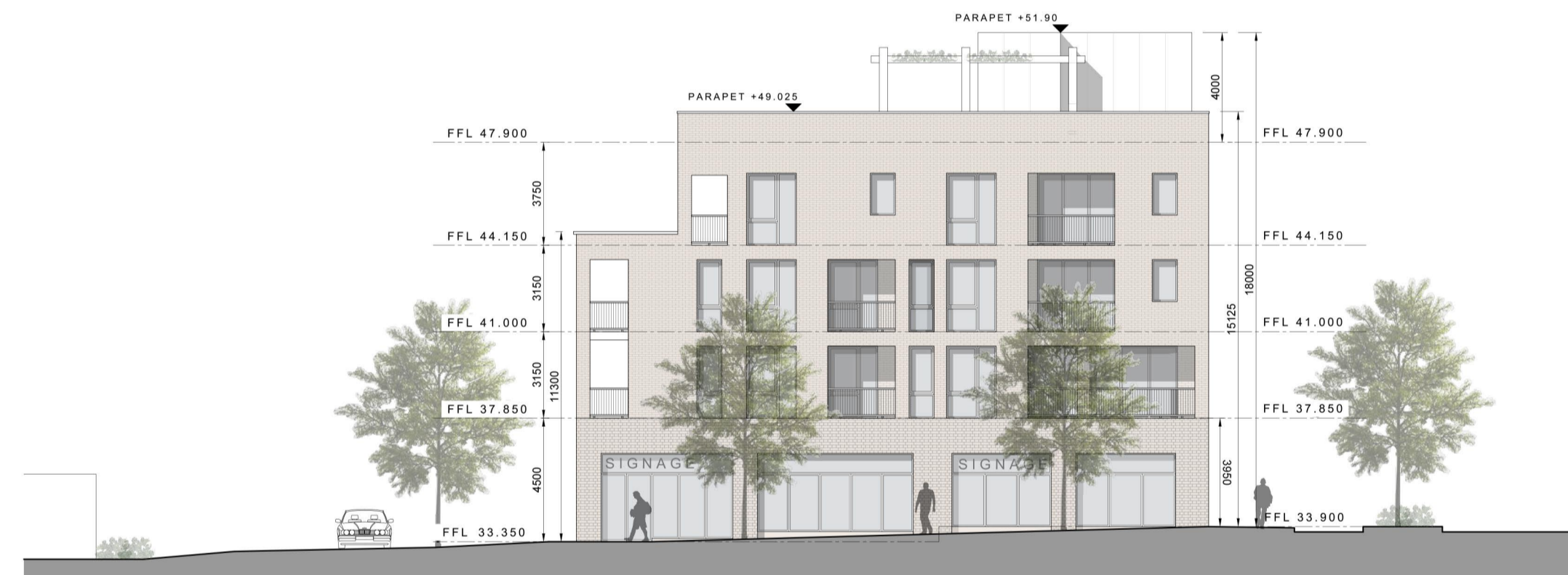
BLOCK D EAST ELEVATION SCALE: 1:200
